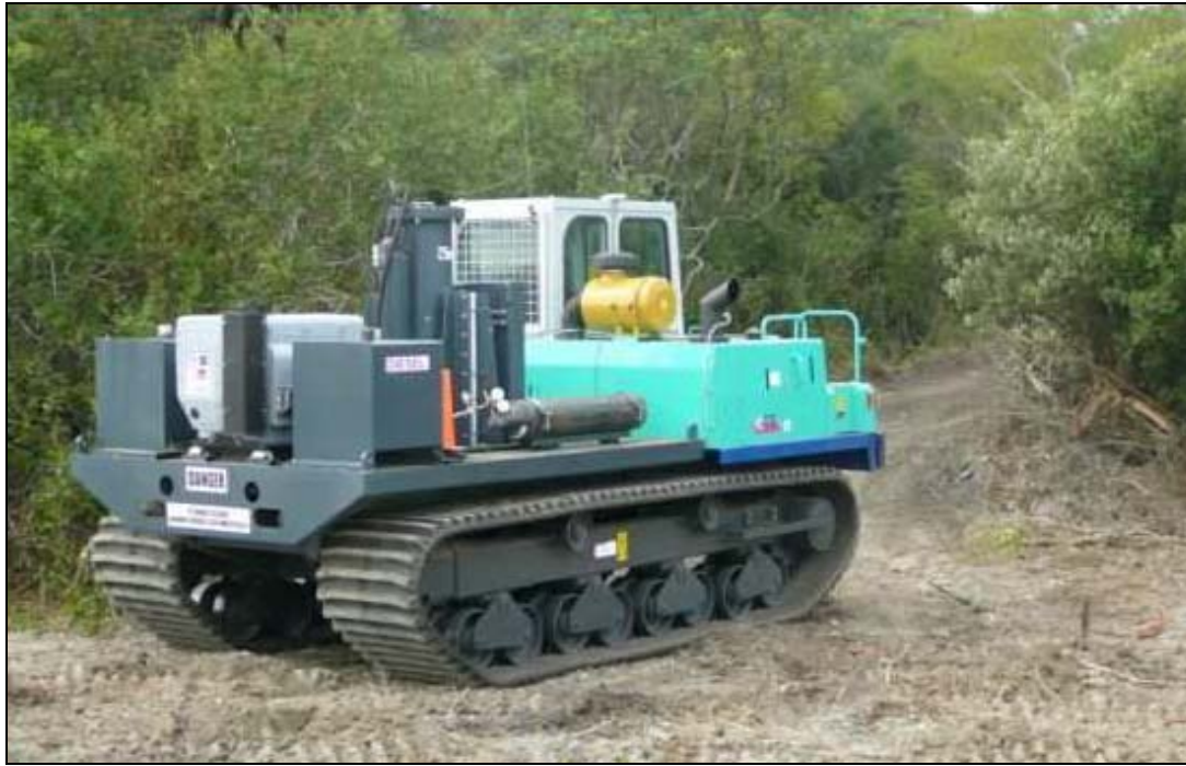
Figure 3 - Crawler-track vehicle with AF750 AIS center mount hammer mass (Geo Survey System, 2014).
