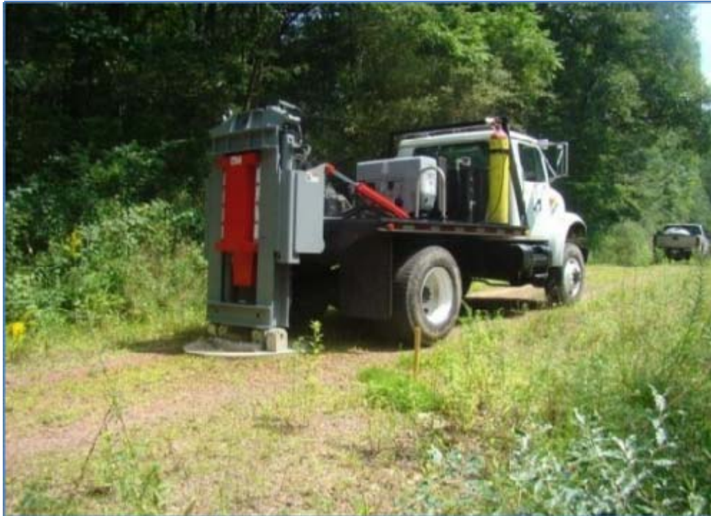
Figure 1 - 4X4 truck mounted AIS system (Geo Survey System, 2014)
